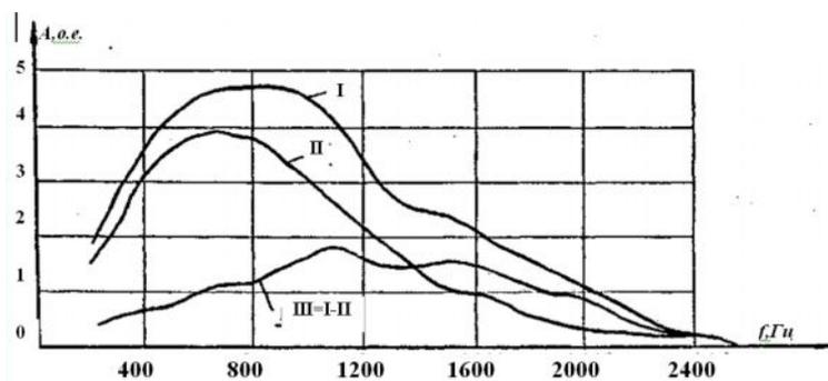
Fig. 3 AFC of the first and second noise chamber at filling with ball load.
