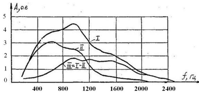
Fig.1 AFC of the first and second chamber noise at filling with ball load.
