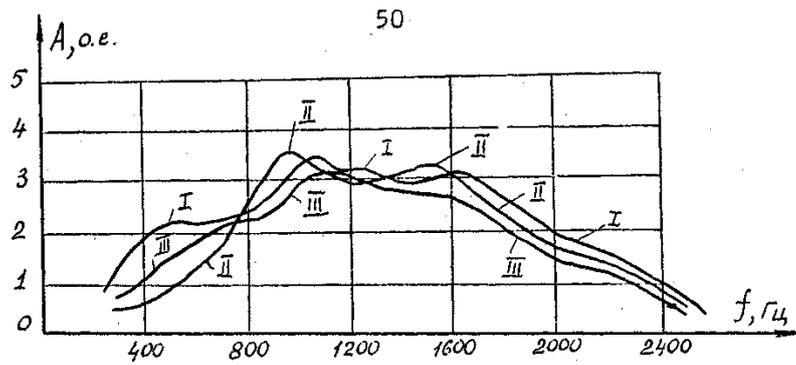
Fig. 4 AFC of connection channel on the mill drum at different ball load:
