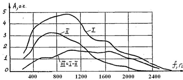
Fig.2 AFC of the first and second chamber noise at filling with ball load.
